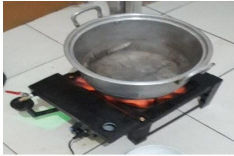
Figure 2. UCO gasification stove when boiling 1 liter of water.
